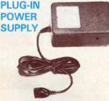
DC Output: +5V @ .9 amp. -5V @ .1 amp. +12V @ .3 amp. Input: 120 VAC/60 Hz., .25A. Coleco #55416
